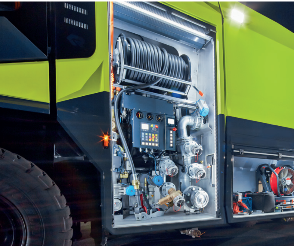
Pump compartment illumination
