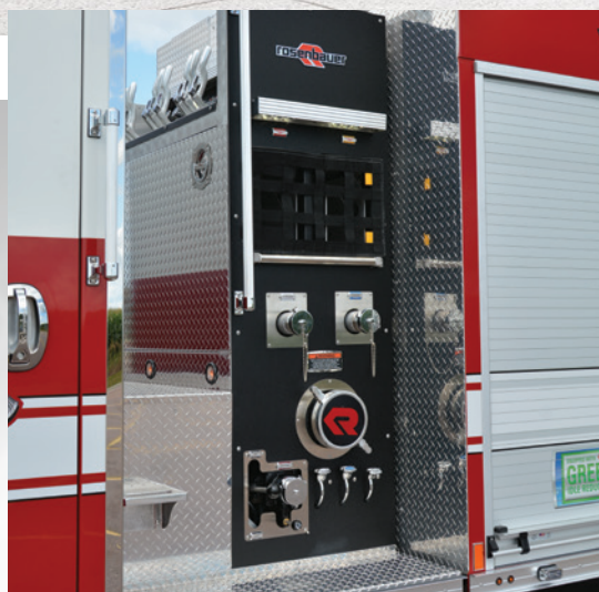
TP3 Pump Control Panel with Sealed Bank
